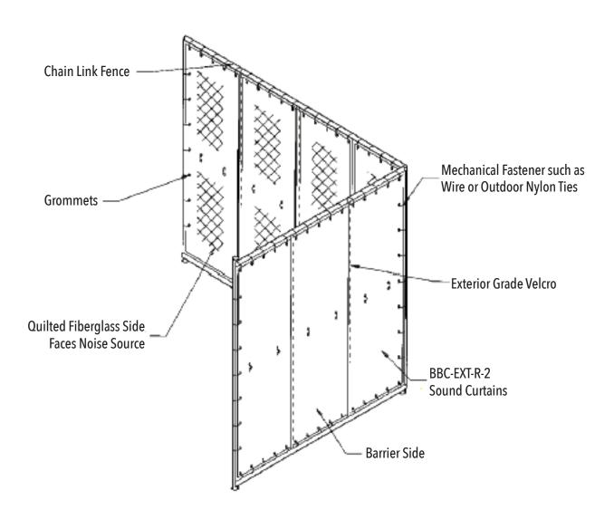
**Detail: Sound Curtain Attached to Chain Link Fence**
