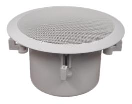
The SMS-SURF is a 25-volt system loudspeaker designed to generate the optimum masking sound for surface-mounted applications. This sound masking speaker is equipped with a 6.5" (16.5 cm) driver installed in a sealed enclosure.
