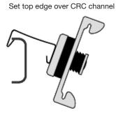
2. Rotate clip around CRC channel
