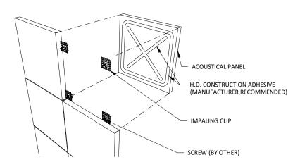
If panels have to be removed, remove old clips and relocate new clips in a different location and repeat installation steps.
