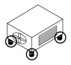
Virtually eliminate structurally transmitted noise and vibration by installing equipment on Spring Mount Vibration Isolators. Properly selected and installed anti-vibration spring mounts offer the greatest assurance that destructive vibration and noise will be eliminated or greatly reduced.
