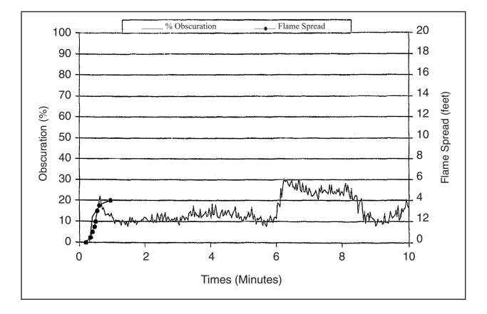
Test Num.: 2 R8078 / I0NK03143 02161008 Flame Spread Index: 20 Smoke Developed Index: 180 Max. Flame Spread (ft.): 4.0
