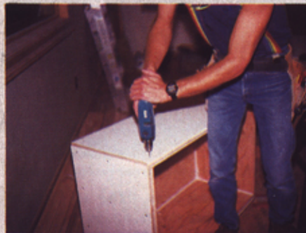
Photo 3: Building the outer speaker enclosures.
