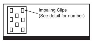
Impaling clips should be applied with long dimension vertically.
