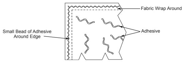
**8.** If panels have to be removed, removal will result in a thin layer of fiberglass adhering to the clips on the wall. Upon replacement of panels in another location locate impaling clips in 2 different locations on panel.
