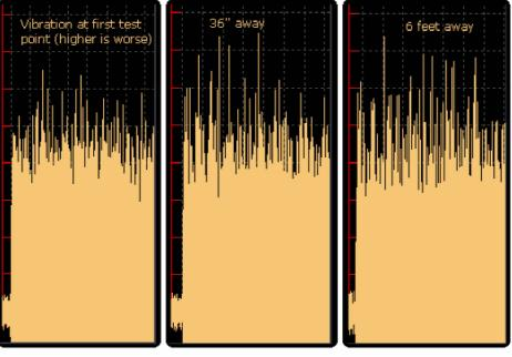
This audio file illustrates the inability of conventional building materials (drywall) to dissipate energy. You hear the decay (lack thereof) over 8 feet in undamped drywall. The level hardly changes, the spectrum merely shifts.
