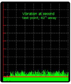
This audio file demonstrates the dramatic noise decay over 8 feet in a Green Glue damped 5/8" drywall panel. The majority of noise in the second segment is simple background noise.
