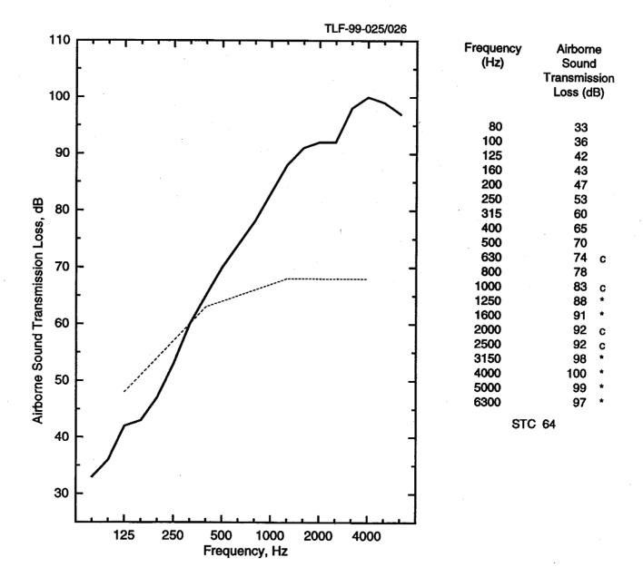
Figure 1: Airborne sound transmission loss measurements of a Specimen B3135-1. The solid line is the experimental data and the dotted line is the STC 64 contour.
