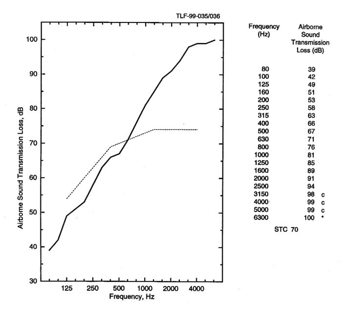
Figure 1: Airborne sound transmission loss measurements of a Specimen B3135-3. The solid line is the experimental data and the dotted line is the STC 70 contour.
