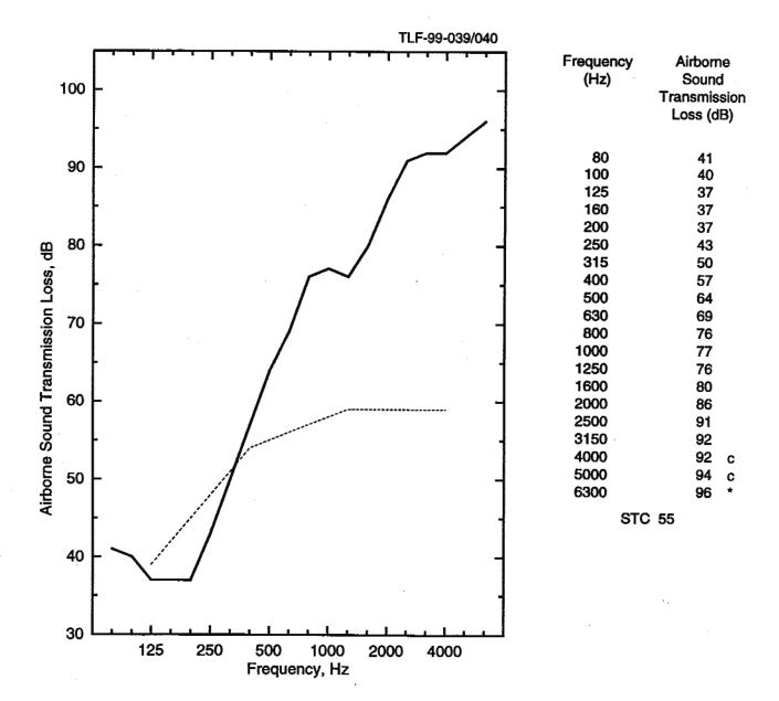
Figure 1: Airborne sound transmission loss measurements of a Specimen B3135-4. The solid line is the experimental data and the dotted line is the STC 55 contour.
