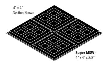
Mini Super W Pads have the same design as Super W Pads but are thinner (3/8"). These rubber isolation pads can be used as noise breaks where the added height of the 3/4" thick Super W is prohibitive. Mini Super W Pads are only made in 45 durometer natural rubber.
