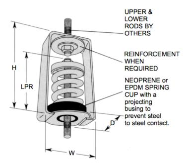
High Deflection Spring Hangers provide far greater vibration control than the lower deflection neoprene hangers. Each powder coated steel spring is in series with a neoprene cup, providing excellent isolation efficiency. The spring serves to isolate a broad range of disturbing vibration frequencies, while the rubber cup is a high frequency or noise break.
