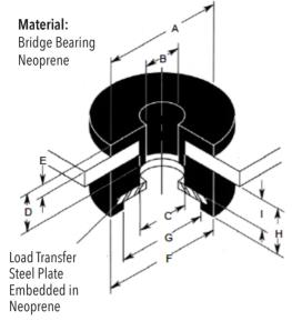
**The HMIB Mounts** – can be used to break the path of vibration. This antivibration rubber mount is an inexpensive way of providing some relief from the noise of a wall fan, a kitchen exhaust fan or a fan assisted strip heater.
