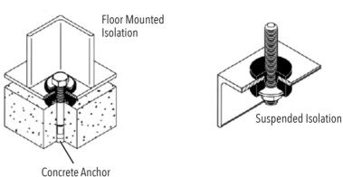
Used for Suspended or Floor Mounted Equipment
